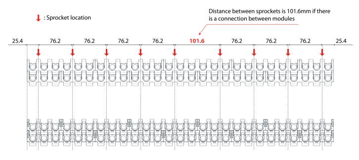
Sprockets are possible every inch (25,4mm) according to the available pockets for sprocket interaction at the opposite side of the belt.
