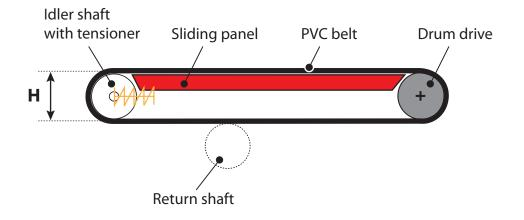
Idler shaft approx. D 30 mm: D as small as possible for short transfers. Drum drive approx. D 80 mm: Depending on required drive data. Tensioner: Spring loaded or manually adjustable. Return shaft: If conveyor is longer than 1 m, shaft every 0,5 m. Sliding panel: UHMWPE or PA or wood.
